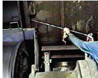
Old Method Spray using graphite, oil, water and solvent
